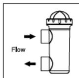
Flow direction marked in the cell must be respected. Recirculation system must guarantee the minimum flow stated in the Table of Technical Specifications for each model.
