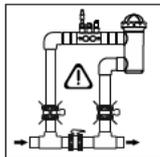
**WARNING:** if the in-out valves of the electrolysis cell are closed simultaneously, the flow detector (gas detector) will not work correctly, with the consequent risk of cell breakdown. Although this situation is extremely unusual, it can be easily avoided once the equipment has been installed, by locking at opened position the return valve to the swimming pool, so it cannot accidentally be manipulated.
